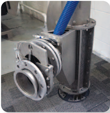
Quick coupling and disconnect flange for ease of installation and removal.
