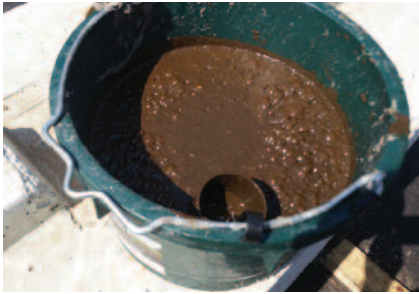
The viscosity of this grease was similar to SAE 30 oil.
