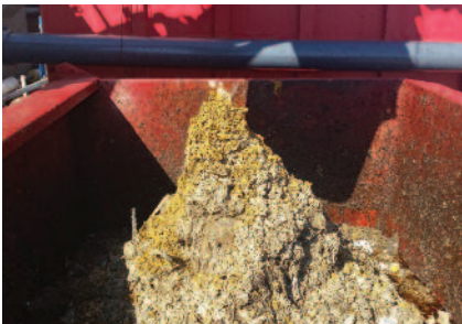
Dry, stackable debris removed from FOG loads.
